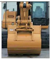
**Bucket Linkage.** Two bucket linkages (CB1 and DB) are available, with lifting eye on the power link.
