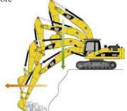
**Truck Loading.** Loading trucks from a bench is more productive and fuel efficient as the return cycle is reduced while the boom down function does not require pump flow.
